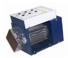
**URM-03/CA** experimental module has been especially designed to provide a comprehensive, hands-on and complete instruction in the principles and operations of AC motor control circuits (drives) most widely used in industry nowadays.
