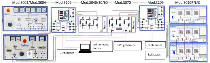
Variable power supply - | -Meter for motor | --motor | generator-- |-Meter for generator |-RLC Loads
