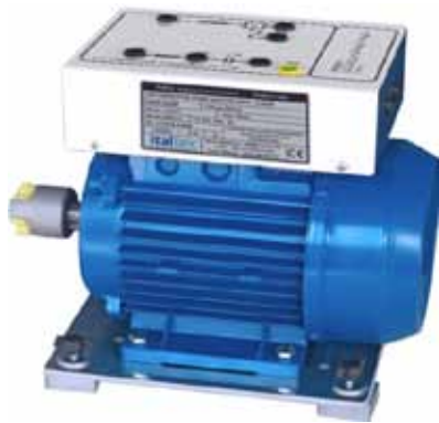
Mod.6122 Single Phase AC Capacitor Start/Cap. Run Motor 2800rpm Mod.6122-4 Single Phase AC Capacitor Start/Cap. Run Motor 1400rpm Single-phase motor with starting auxiliary phase, complete with starting switch and starting and running capacitor
