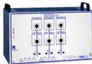
Mod.3020-110R Load resistive for dynamo and 3-phase alternator; Starter for DC motor.; · Variable 3x 1%÷110%; · 3Ph: variable with 110 steps from 1% to 110% · Power: 5÷550VA; · Monophase: with 330 steps 1,6÷550VA
