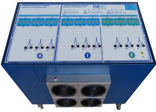
Robust sheet metal steel painted in the oven, mounted on four robust swivel wheels for easy movement.
