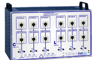
Mod.6020T-110LC Charge for triphase alternator • Inductive & capacitive load variable with 3x 1%÷110%; • 3Ph: variable with 110 steps from 1% to 110% • Power: 30÷3000VA; Triphase / monophase; (monophasé with 330 steps);
