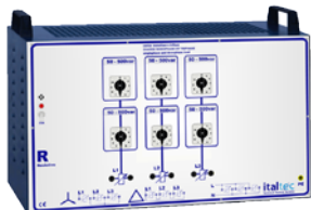
Mod.6020T-20R Load resistive for dynamo and alternator; Starter for DC motor; Speed control for slip-rings motor; • Variable load 3x5÷100%; • Power: 150W÷3000W 3-phase/ single-phase;
