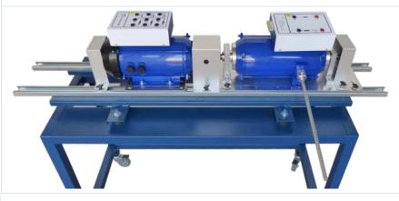
The machines of this system can be supplied with a suitable base that allows an easy and safe coupling with other machines. It is fast and easy to realise groups of machines.
